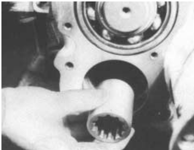
2. Fit the adaptor coupling onto the rear of the left-hand countershaft.
