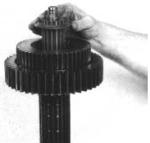
7. Fit the 3rd gear assembly clutching teeth up, selected graded mainshaft washer and snap ring.
