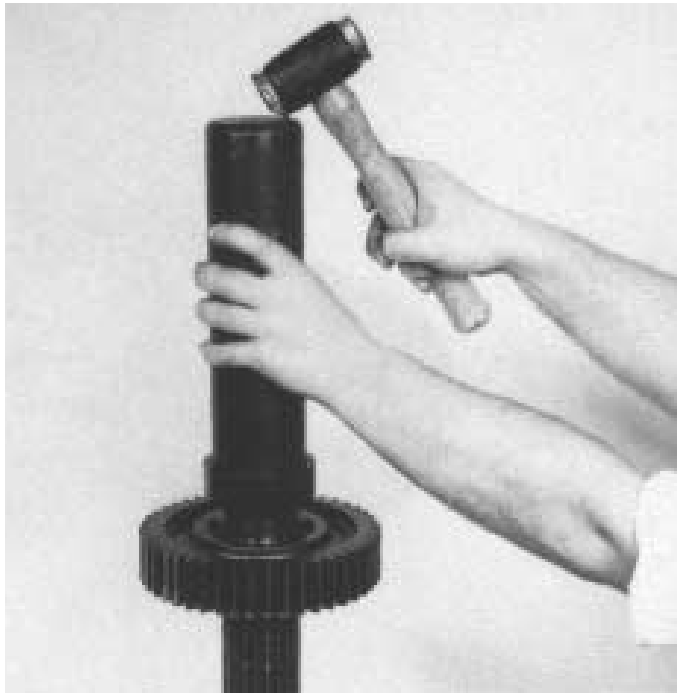
4. Press the 2nd/3rd gear spacer onto the shaft.
