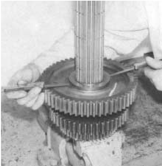
16. Check the clearance between 1st speed gear and the washer using two sets of feeler gauges. If the clearance is not within the correct limits the graded washer should be removed again and a thicker or thinner graded washer installed as required in its place.
