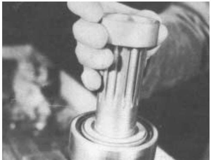
4. Fit the spacer sleeve.
