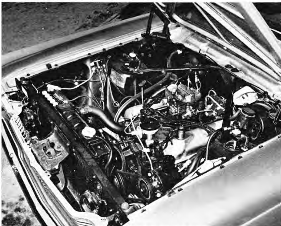
ENGINE WITH 2-barrel carburetion imparts average performance to the Fairlane but 3-speed automatic transmission makes best use of power available.
