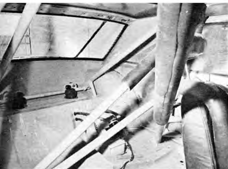
FOUR SHOCK absorbers attach to rear roll cage crossmember. Blower/cooler on floor keeps rear axle lubricant cool.
