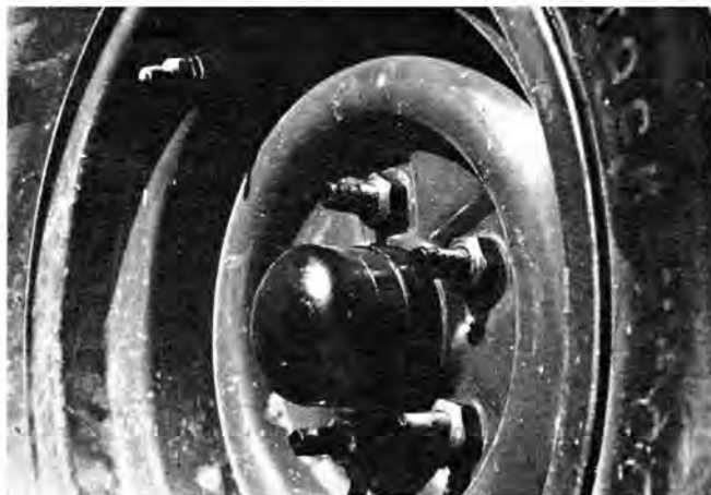
LARGE-DIAMETER , extra-long wheel studs, huge wheel bearing cups reflect magnitude of stresses absorbed in racing.
