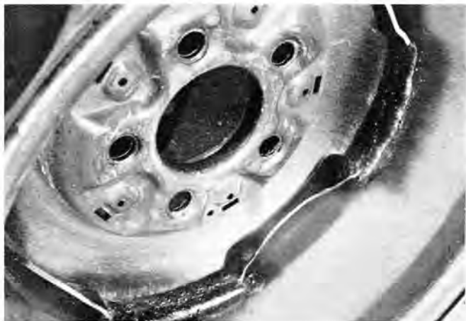
STEEL WHEELS have double-thickness center sections to prevent lug nuts from pulling through wheel during hard cornering.
