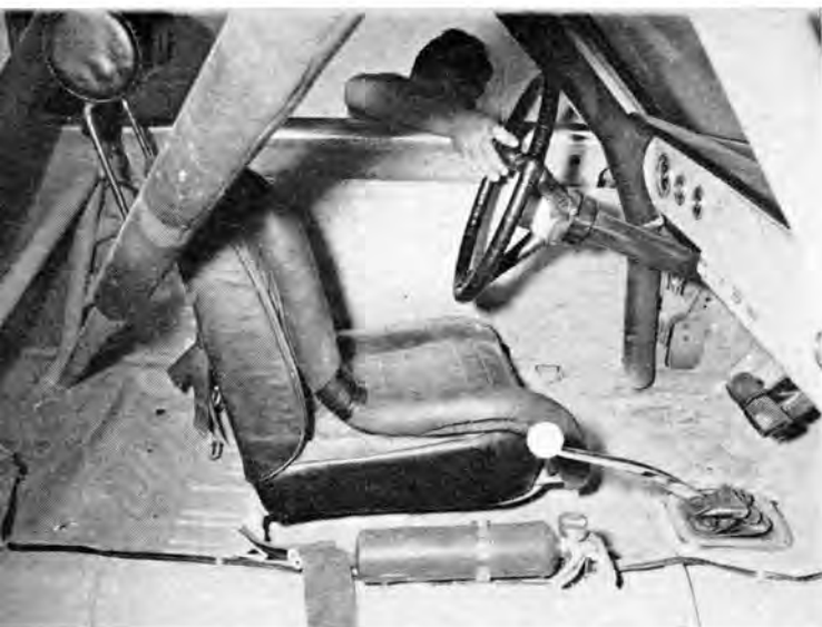
RICHARD'S ROOST features seat bolster to combat centrifugal force in left turns, padded steering wheel and headrest.
