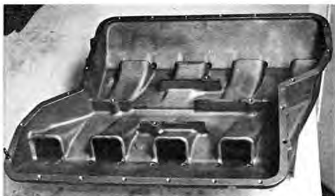
RAM-TUNED intake manifold offers 20-bhp gain over conventional manifold shown in engine photographs, but throttle response is poor, causing driving problems on short oval or road courses.
