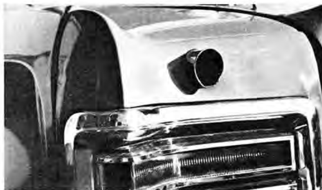
FUEL TANK is safely encased by rear sheet metal, carries 4-in. diameter, straight-flow filler tube and 1-in. vent tube which exits just above left rear taillight through fender cap assembly.
