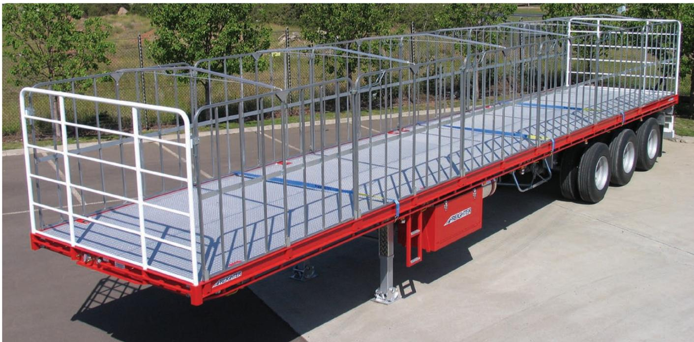
The Freighter Flat Top Semi-Trailer may be purchased as a tailored, stand alone trailer or in tag specification to use with an existing lead trailer for maximum payload flexibility.
