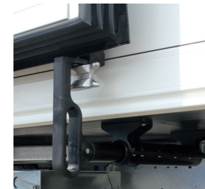
The pivoting handle ensures the safe and easy catching of the doors, close to the sidewalls.
