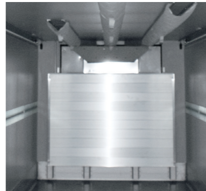
The air circulation wall on the front bulkhead ensures an energy-efficient flow of air. Flexible cooling ducts for the distribution of cold air. (Optional)
