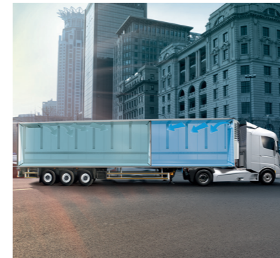
Multi Temp Zones with exact temperature settings. (Optional)
