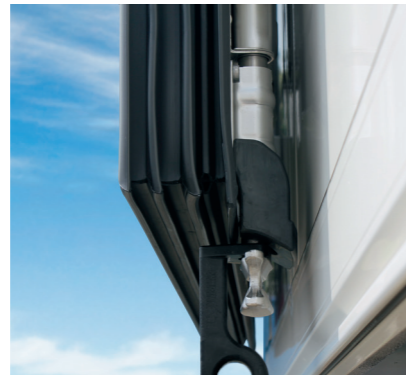
Four lip door seals perfectly protect the trailer from the loss of cold.
